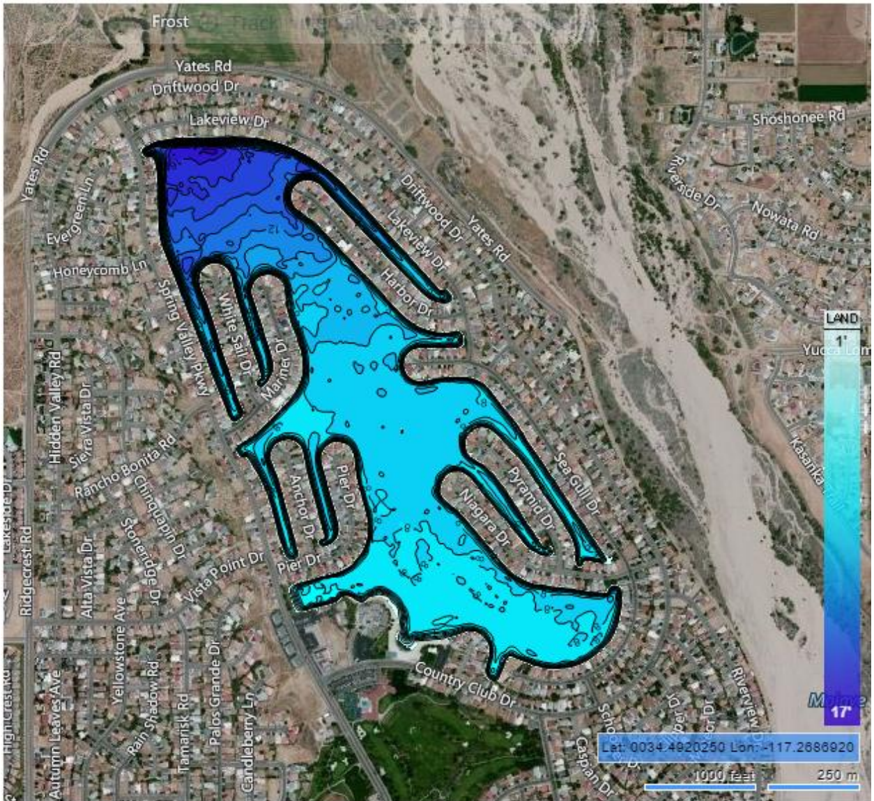
This image shows the current bathymetry of Spring Valley Lake. Slight changes have occurred since the previous spring.
