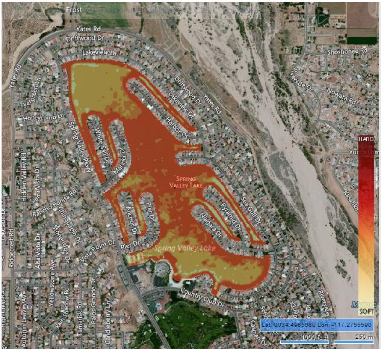
This map shows the current bottom hardness present in the lake. The legend bar on the right shows the graduated scale.
