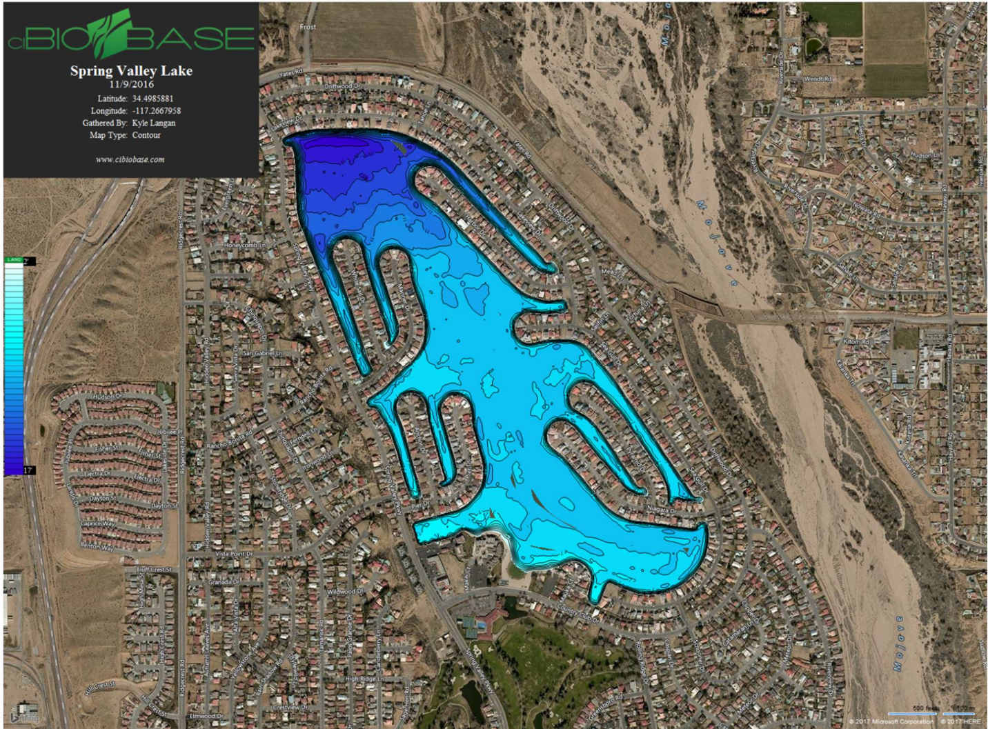
This image shows the current bathymetry of Spring Valley Lake. Almost no change was detected since the previous mapping earlier this spring.
