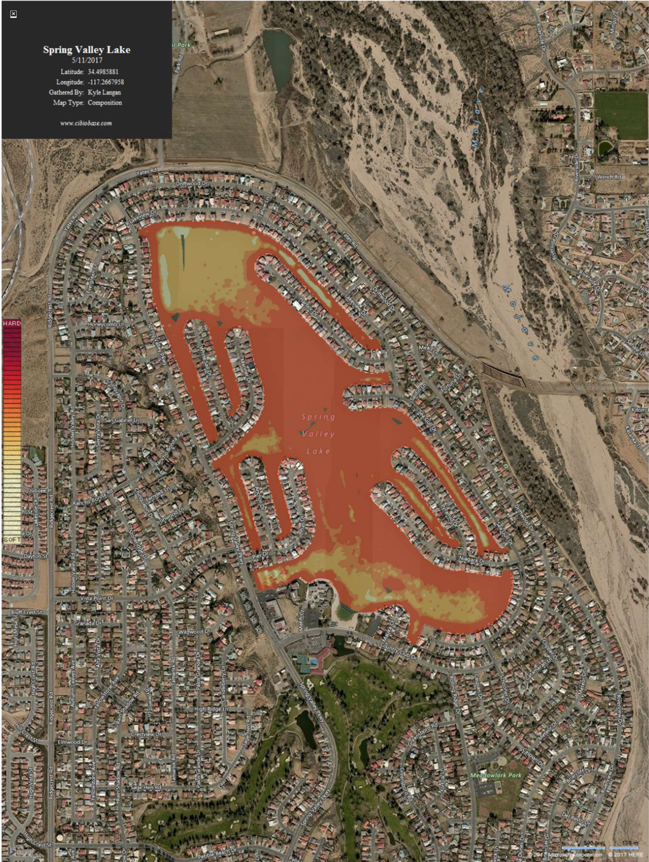
This map shows the current rd bottom hardness present in the lake. The legend bar on the right shows the graduated scale.
